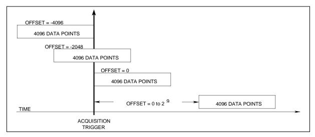
Figure 7-7. Pre-trigger and Post-trigger Acquisition
